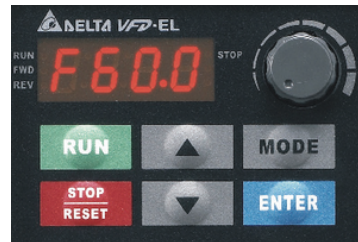
Figure 3: VFD control panel
