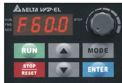
Figure 2: VFD control panel
